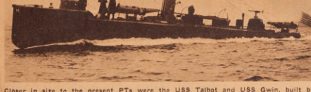
Closer in size to the present PTs were the USS Talbot and USS Gwin, built by Herreshoff in 1897. The boats were of steel construction, 100 feet overall and drew five feet, three inches. They were designed with a plumb stem and stern, had a flat raised deck forward of the conning tower. The vessels turned up a speed of 21 knots.
