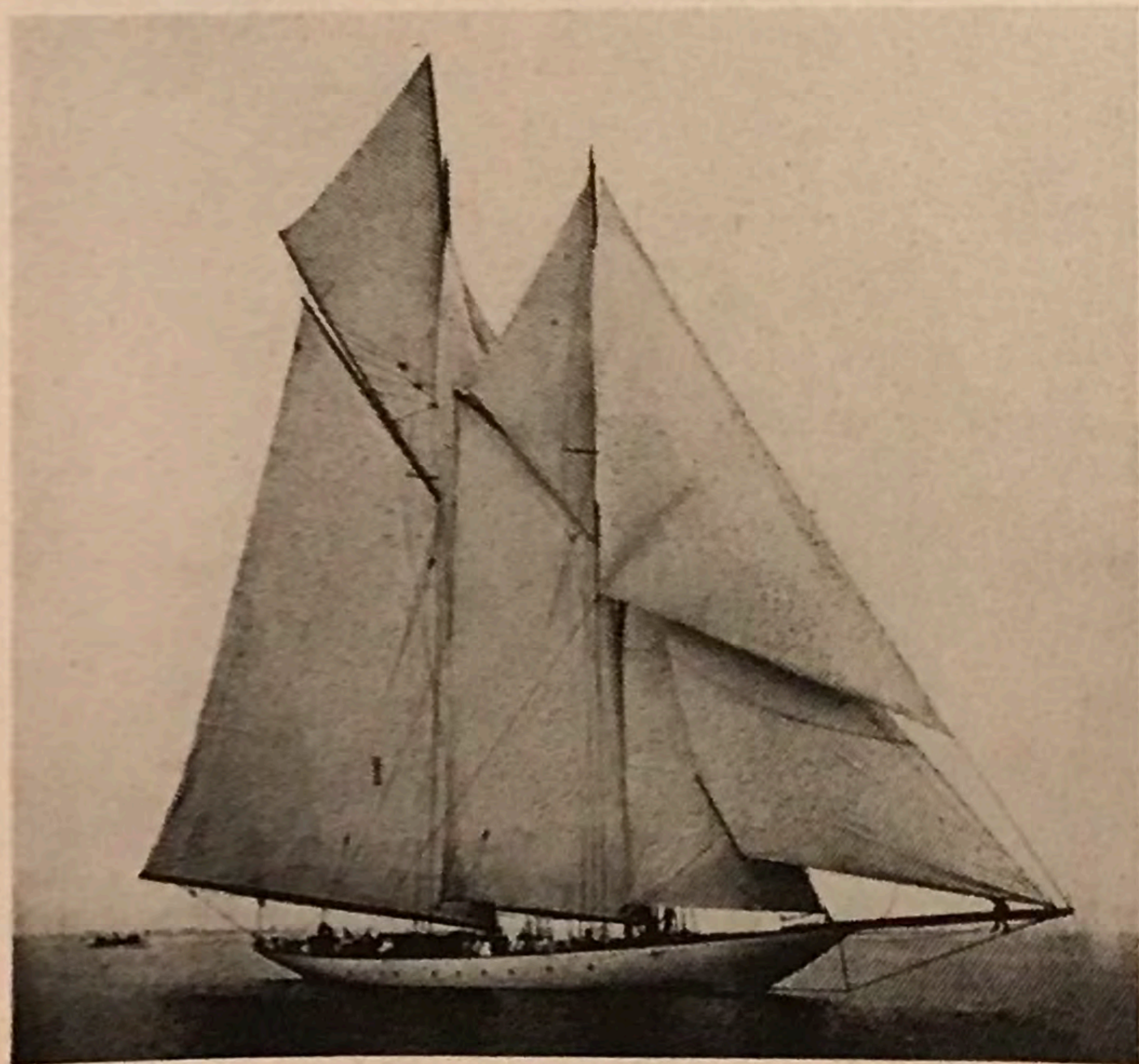
Fig. 86. Corona (ex-Colonia) rigged as a schooner
